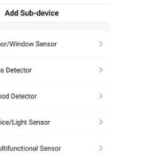
3/ Press and hold the sensor's reset button for more than 5 seconds, until the network indicator LED begins to blink. Then, follow the instructions on the app to add the device.
